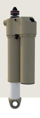
Developed by Horstman in the late 1980s for tracked vehicle and wheeled applications, Hydrostrut® was designed from the outset to eliminate the need for a separate spring by combining the gas spring into the damping unit. This allows the vehicle designer to overcome internal packaging constraints in the case of torsion bars or external packaging constraints in the case of coil springs.
