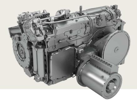
The HSWL 256 EVO transmission offers superior maneuverability due to the 6 speed transmission and high performance steering system with true pivot functionality. The system features the M82 electric motor generator, providing additional mobility and power generation capabilities to the vehicle platform. The HSWL 256 EVO also includes Drive-By-Wire functionality.
