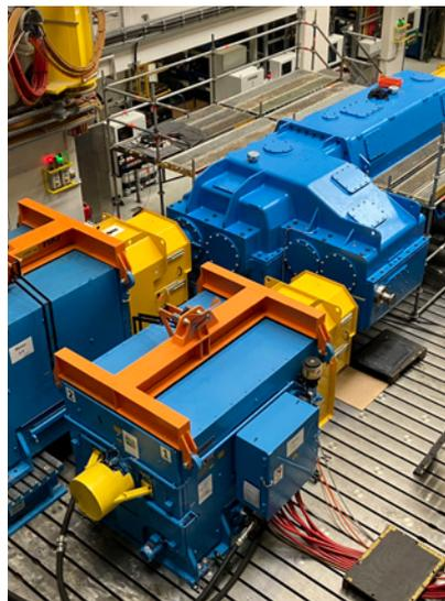
RENK's multifunctional testing facility with lifting capabilities up to 240 tons and test power up to 12 MW is located at RENK Group headquarters in Augsburg, Germany.
