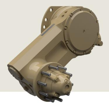
Developed by Horstman in the mid-1990s, InArm® is designed to eliminate the need for torsion bars and to minimize or eliminate road arm penetration of the vehicle hull.
