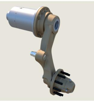
Developed by Horstman in the 1970s for the UK MOD Warrior Infantry Fighting Vehicle (IFV) requirement, rotary damper suspension provided an upgrade in performance and reduced external space claim over linear shock absorber solutions.
